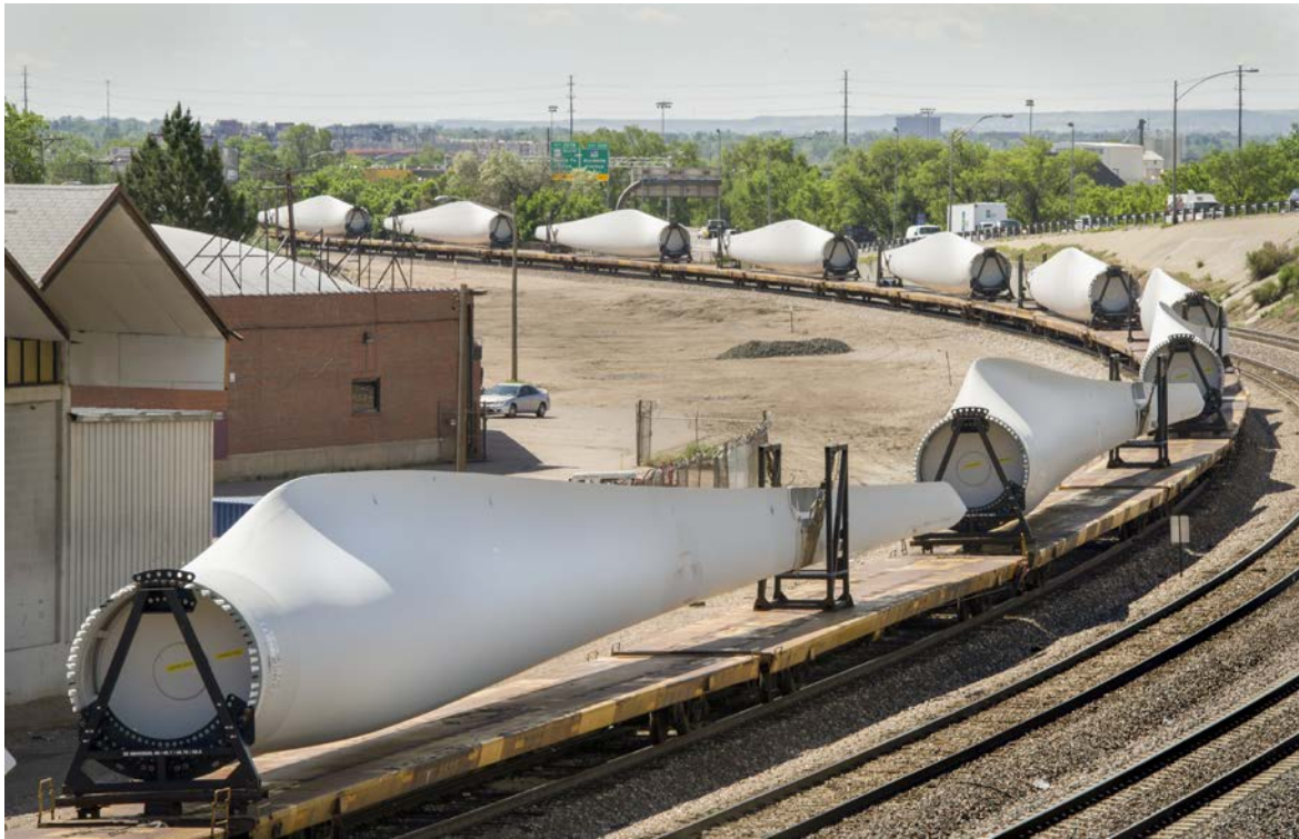
Wind turbine blades wind their way by train through Denver, CO (Photo credit: US Department of Energy/Dennis Schroeder/NREL)
