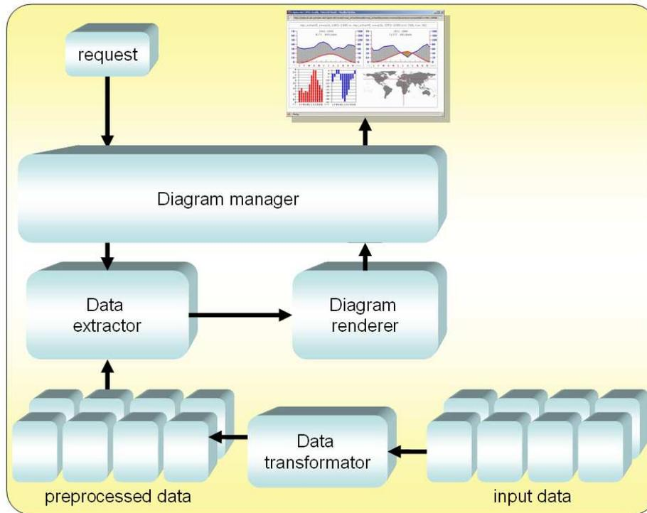
Fig. 9 – Diagram server architecture
